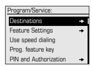
The menu structure comprises several levels. The first line in this structure shows the menu currently selected while the second line shows an option from this menu. An arrow next to an entry indicates additional options for this entry.
