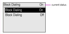
An example of the display during en-bloc dialing is on  $\rightarrow$  Page 24. For a description of en-bloc dialing, see  $\rightarrow$  Page 50.
