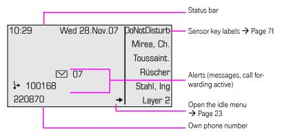
The left area contains the status bar on the first line, followed by a five-line field for additional displays. ?
