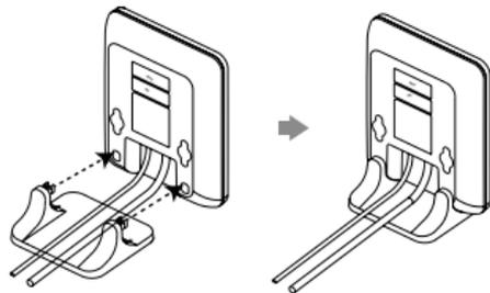
Align the snap-fits with the corresponding holes and push forward, snapping them into the holes.
